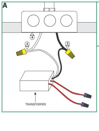
**NOTE:** Use the universal round crossbar (provided) if the electrical box holes are not spaced 2-3/4" apart.
