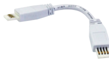
Interconnection Cable NAL-802W 2" Cable NAL-806W 6" Cable NAL-812W 12" Cable NAL-824W 24" Cable NAL-872W 72" Cable Used to join two fixtures together or to in-line dimmer or motion sensor.
