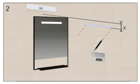
4. Drill and insert the screw anchors suited to the type of wall to which the cabinet mirror will be fixed (only screws in the case of wood studs) and install the fixing bar with its screws as shown.
