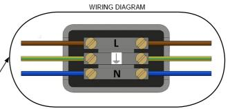
6. Connect the mirror wiring in an IP44 approved connector box (not included) which can be inserted into the wall anywhere behind the mirror.
