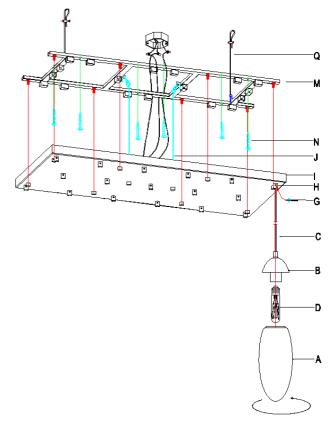
In Instruction: This fixture is provided with a Safety Cable. The Safety Cable provides a back up system the mounting frame and the installation hardware. It is essential that the Safely Cable be properly installed. The Cable must be secured to a STRUCTURAL MEMBER of the building, and not to the outlet box. The Cable must be terminated with Steel cable lock kit specifically sized for the Cable per the following steps:
