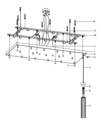
In Instruction: This fixture is provided with a Safety Cable. The Safety Cable provides a back up system the mounting frame and the installation hardware. It is essential that the Safely Cable be properly installed. The Cable must be secured to a STRUCTURAL MEMBER of the building, and not to the outlet box. The Cable must be terminated with Steel cable lock kit specifically sized for the Cable per the following steps:
