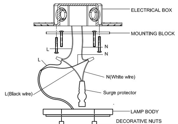
Note: It is recommended that each surge protector be connected to a maximum of 6 LED boards!
