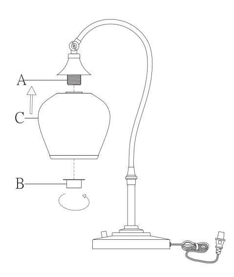
Socket ring(B) comes pre-assembled to the socket. Before assembling the shade, please unscrew this socket ring(B). Set shade(C) onto socket(A) and tighten clockwise with socket ring (B) to secure shade.
