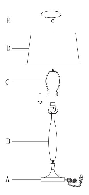
1. Screw part(B) clockwise into base(A) to tighten.
