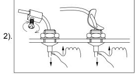
Step.2: Press the wire restraint to adjust the desired length of cable and secure the cables and wire with lock and screws.
