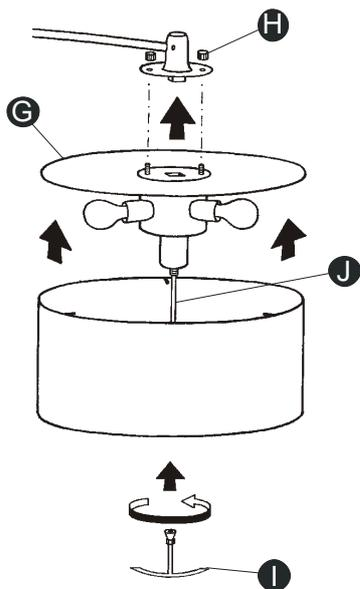
6. Connect the fixed lamp support (G) set into the arms socket and tighten with the nuts (H). Fix the lamps and the screen. Introduce the hilt (I) into the axle switch (J) and tighten it to a firm support.
