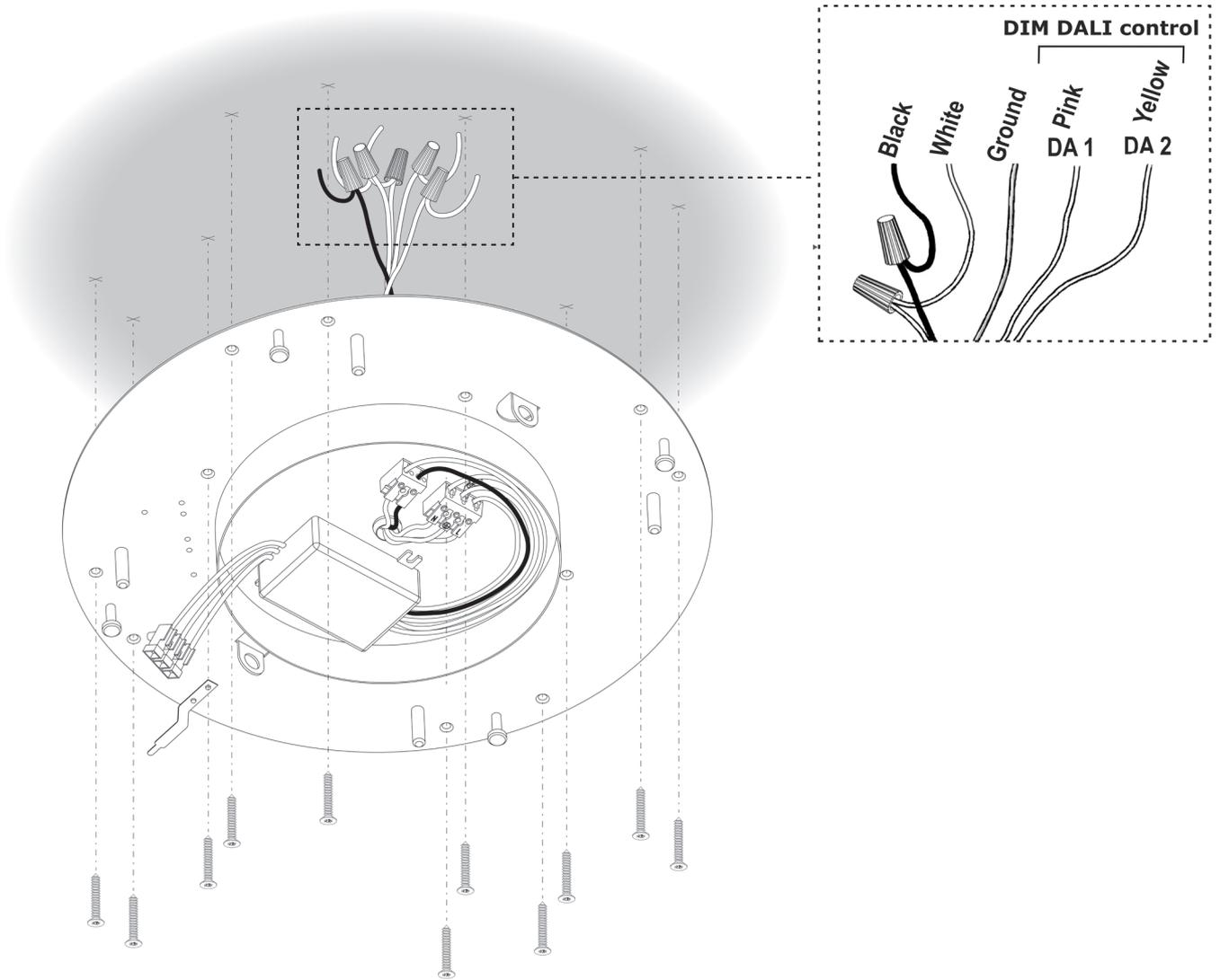
**IMPORTANT:** If you have ordered a fixture with a driver specifically compatible with DALI DIMMING SYSTEM. This fixture will not be compatible with other types of dimming systems. You can check you have the correct product by looking at the model number printed on the box label or fixture canopy finished in 11 or 41: XXXX-XX/11, for example: 4870-18/11.
