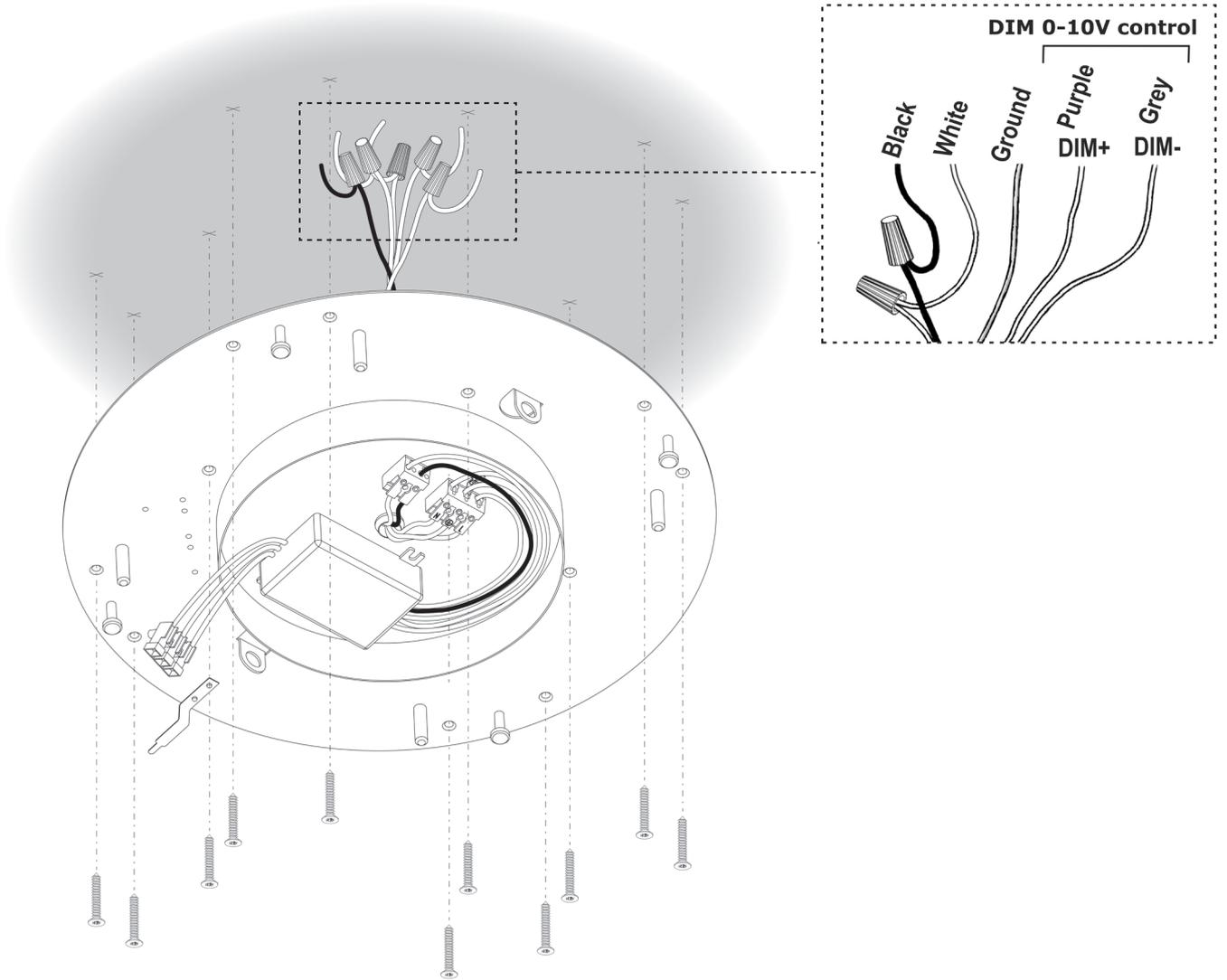
**IMPORTANT:** If you have ordered a fixture with a driver specifically compatible with 0-10V DIMMING SYSTEM. This fixture will not be compatible with other types of dimming systems. You can check you have the correct product by looking at the model number printed on the box label or fixture canopy finished in 12 or 42: XXXX-XX/12, for example: 4870-18/12.
