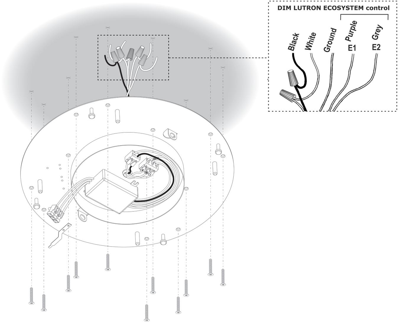
**IMPORTANT:** If you have ordered a fixture with a driver specifically compatible with LUTRON ECOSYSTEM DIMMING. This fixture will not be compatible with other types of dimming systems. You can check you have the correct product by looking at the model number printed on the box label or fixture canopy finished in 17 or 47: XXXX-XX/17, for example: 4870-18/17.
