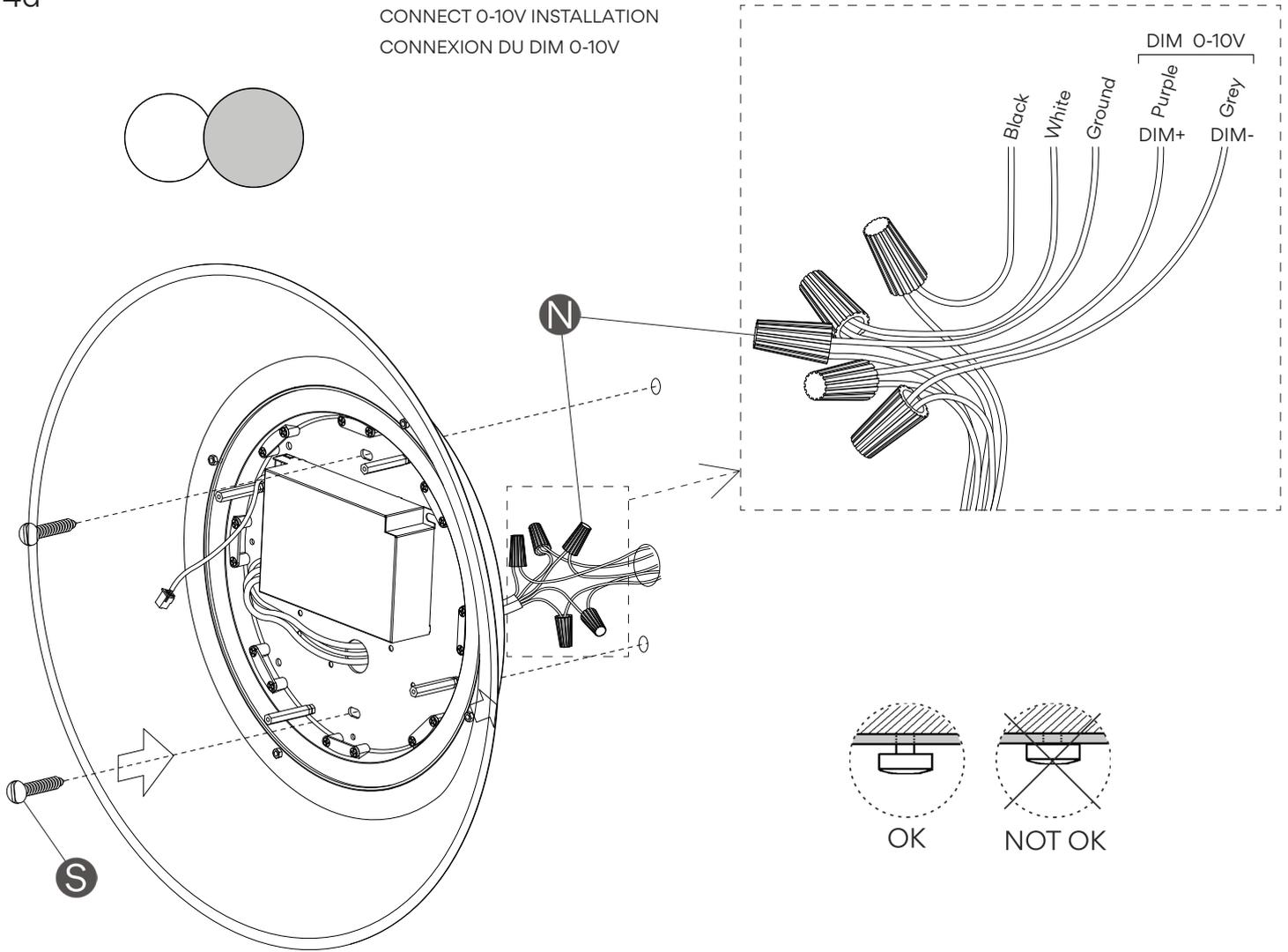
**IMPORTANT:** You have ordered a fixture with a driver specifically compatible with 0-10V DIMMING SYSTEM. This fixture will not be compatible with other types of dimming systems. You can check you have the correct product by looking at the model number printed on the box label or fixture canopy finished in 12: XXXX-XX/12, for example: 5481-72/12.
