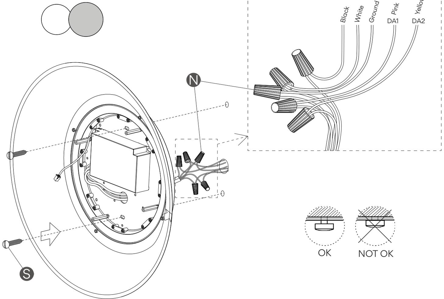
**IMPORTANT:** You have ordered a fixture with a driver specifically compatible with DALI DIMMING SYSTEM. This fixture will not be compatible with other types of dimming systems. You can check you have the correct product by looking at the model number printed on the box label or fixture canopy finished in 11: XXXX-XX/11, for example: 5481-72/11.
