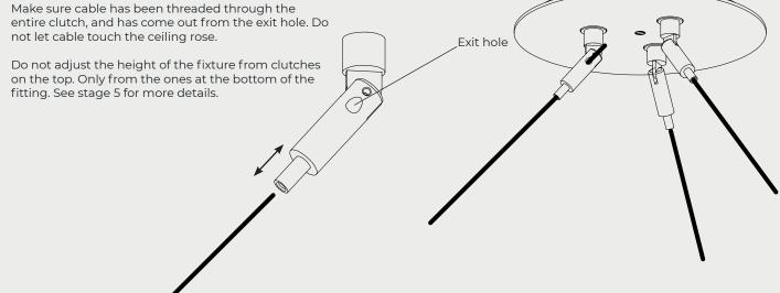
2. Install the body making sure to align positive (+) clutch to positive clutch and negative (-) to negative. Each clutch will be marked with a small removable label.
