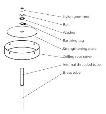
**T**. Fix the mounting plate to the ceiling. Ensure that suitable screws are being used for the surface that you are mounting to (not supplied).
