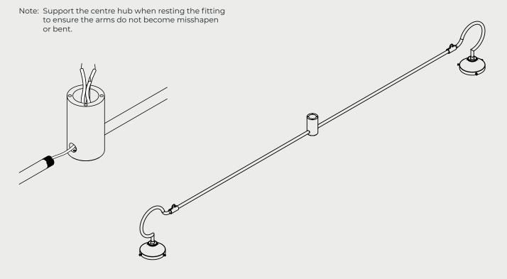
2. After the arms have been screwed in, neatly join the same coloured cables to each other inside the central hub. Ensure that the colours match:
