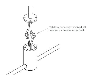
Carefully push the loose cables into the centre hub and close the centre hub cap over the connections.
