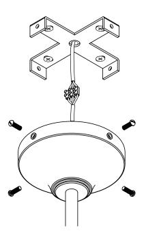
7. With the pendant secured to the ceiling, adjust the rotation of the arms to ensure they are all sitting straight with the bulb holders facing straight down and tighten 4.no Hex Key screws located underneath the central hub to secure the arms in place. Screw central hub bottom cover by hand onto the underside of the hub to hide screw fittings.
