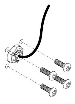
6 . With the base securely fixed to the bottom of the stem, clamp the cable to the base using the supplied clamp and screws.
