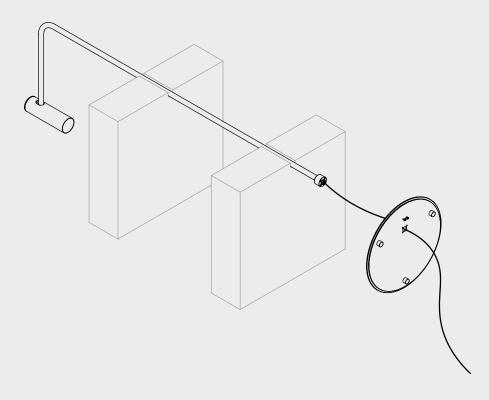
**5**. With the base positioned on the end of the stem in the correct orientation, secure with the 4 x screws.
