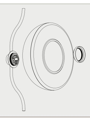
6. Thread the diffuser (F) into the body (C).
