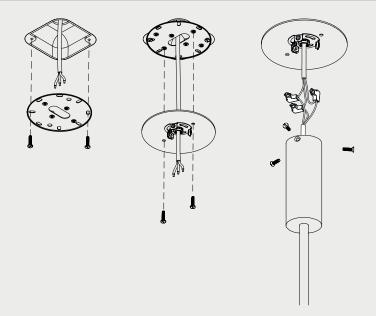
Cable the transformer (G) into the 2 core cable and the 3. mains from the ceiling.
