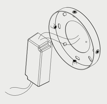
3. Attach the wall mount onto the wall plate.
