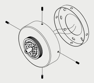
4. Place the Glass shade (B) onto the wall mount (A) and fix into position by threading on the Glass mount ring (C).
