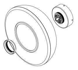
**5**. Thread the diffuser into the wall mount (A).
