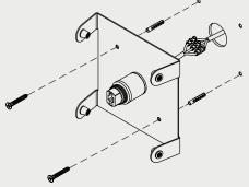
1. US Make the electrical connection inside the junction box.
