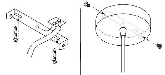
**6** Adjust the cable. Screw the support bar into the ceiling, connect the cable to the power supply, and fasten the ceiling rose using the two screws. Plug a LED bulb E26. We recommend having this step done by a professional if you don't feel confident in handling the electrical system.
