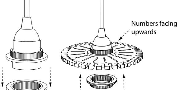
**1** Unscrew the lower tightening ring of the socket. Insert the socket into the numbered gearwheel (a.1) and screw the ring back in place. Tighten both rings to securely hold the numbered gearwheel (a.1) in place.
