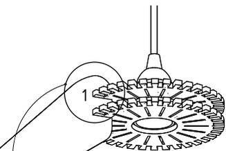
**3** Insert the slat #1 into both gearwheels, following the instructions of last step.
