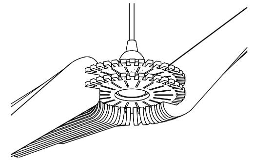
Keep inserting slats (b) by following the numbering until you complete the assembly.
