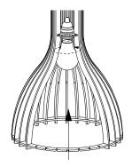
Screw a LED bulb E26 into the socket.
