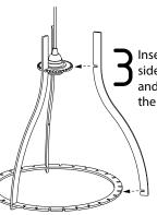
Insert a slat (b) on the two opposite sides in order to stabilize the model and facilitate the remainder of the assembly.
