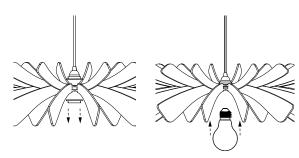
Unscrew the lower tightening ring of the socket. Insert the socket into the gearwheel (a.1) and screw the ring back in place. Tighten both rings to securely hold the gearwheel (a.1) in place.
