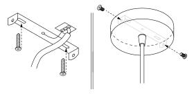
Adjust the cable. Screw the support bar into the ceiling, connect the cable to the power supply, and fasten the ceiling rose using the two screws. Plug a LED bulb E26. We recommend having this step done by a professional if you don't feel confident in handling the electrical system.
