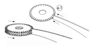
Insert the upper notch of a large slat (b) into the gearwheel (a.1), then the lower notch into the other gearwheel (a.2). The slat must be oriented downwards, this applies to all large slats.
