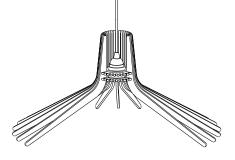
In this way, we continue to fit the slats one by one around the wheels and ensure that each slat is properly engaged.
