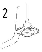
Next, fit the second wheel onto this slat. If the socket obstructs the fitting, raise it until there is enough clearance for wheel (a.2).
