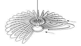
Keep inserting slats (b) until you complete the assembly.
