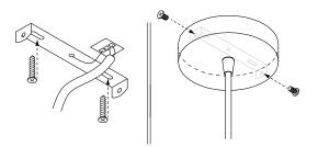
Adjust the cable. Screw the support bar into the ceiling, connect the cable to the power supply, and fasten the ceiling rose using the two screws. We recommend having this step done by a professional if you don't feel confident in handling the electrical system.
