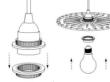
Unscrew the lower tightening ring of the socket. Insert the socket into the big gearwheel (a.2) and screw the ring back in place. Tighten both rings to securely hold the gearwheel (a.2) in place. Plug a LED bulb E26 into the socket.
