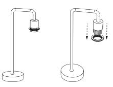
Screw the mast of the stand onto its base, then unscrew the clamping ring of the socket.
