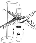
Insert Alba into the socket of the stand, then tighten the clamping ring.
