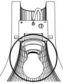
Tighten the ring to lock the model onto the bracket and screw in the light bulb.
