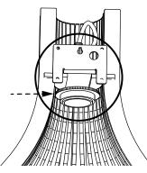
The top wheel should fit between the metal bracket and the ring.
