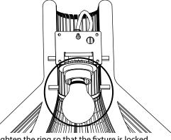
Tighten the ring so that the fixture is locked onto the bracket, then screw in the light
