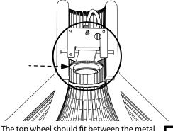
The top wheel should fit between the metal bracket and the ring.
