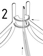
Continuing to ensure both notches are engaged simultaneously, repeat the operation until the entire model is assembled.
